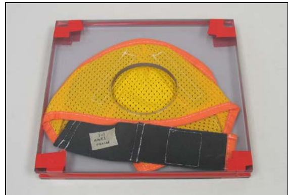
Figure 2: Mask with filter attached for Filter test
