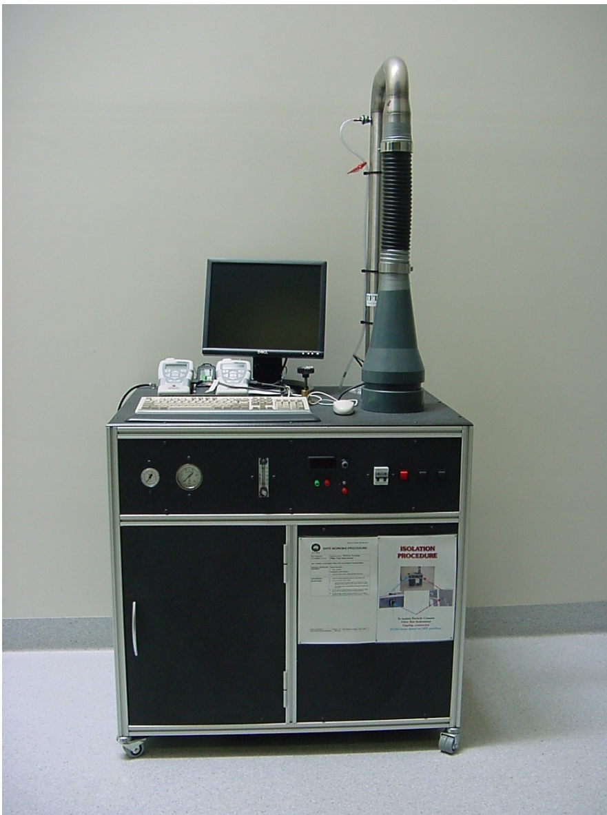
Figure 3: Image of the Particle Counter Filter Test Instrument (PCFTI) with HandiLaz Particle Counters.
